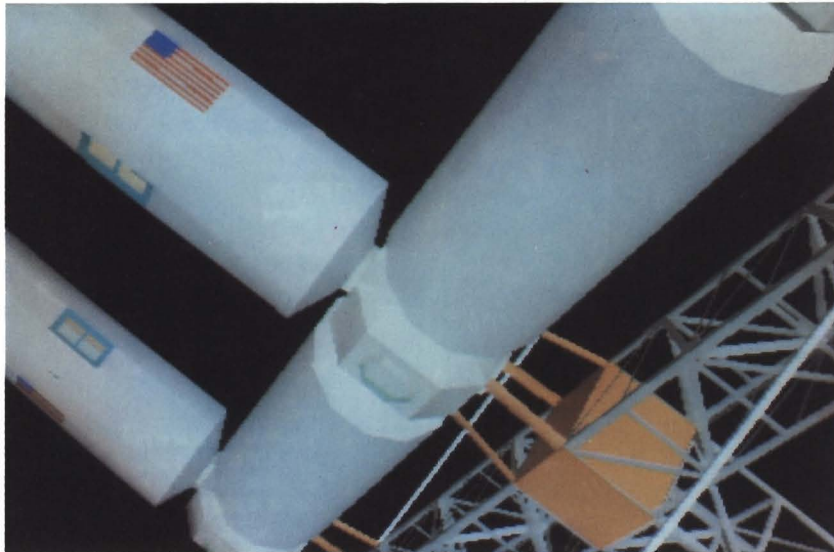
Photograph 3a) and b): Polygonal image before ( top ) and after ( bottom ) anti-aliasing. Non-antialiased image updated at 8 frames per second; anti-aliased image generated in about 6 seconds after user releases input devices. Speed penalty is equal to the number of sub-samples taken. A non-antialiased image is produced as the image moves, but when the image becomes static the super-sampling algorithm is applied in successive refinements (with an increasing number of sub-pixel samples). Database courtesy of Don Eyles.
