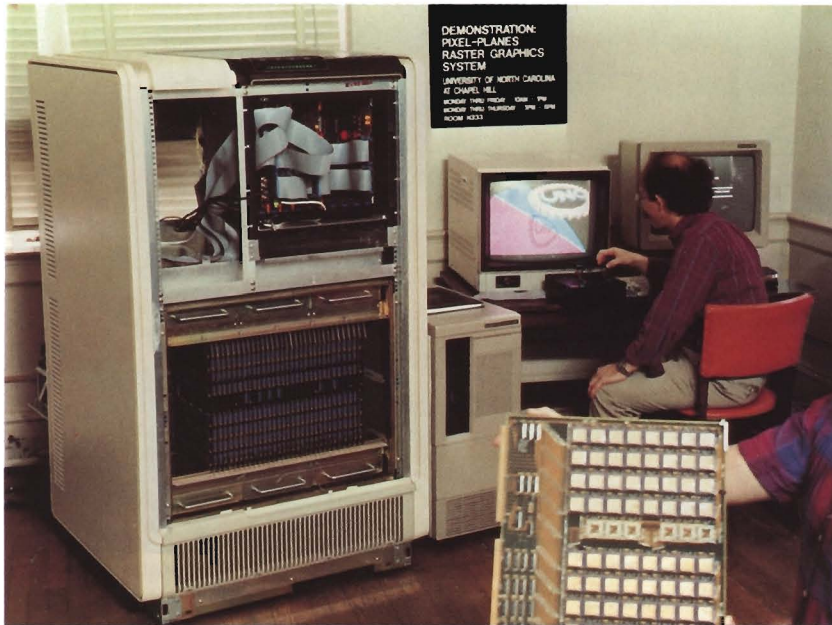
Photograph 1: Pixel-planes graphics system. Cabinet containing custom hardware on the left small upper rack contains Graphics Processor, Image Generation Controller, and Video Controller; large lower rack contains 2048 logic-enhanced memory chips. Host and Pixel-planes monitor are on the right with PI Henry Fuchs manipulating joysticks.
