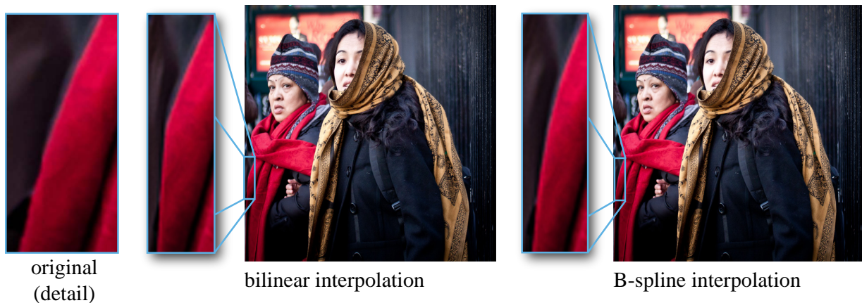
Figure 3.36: Images of high resolution may benefit from higher-order interpolation when using coarse grids for the retargeting optimization. Here we show an example where the input image resolution is 2800 \times 1800 and the retargeting uses a 25 \times 25 grid. Bilinear interpolation on this grid leads to some smoothness artifacts (middle), while upsampling to a 100 \times 100 grid using the spline technique described in Sec. 3.4.4 results in visually smooth interpolation.
