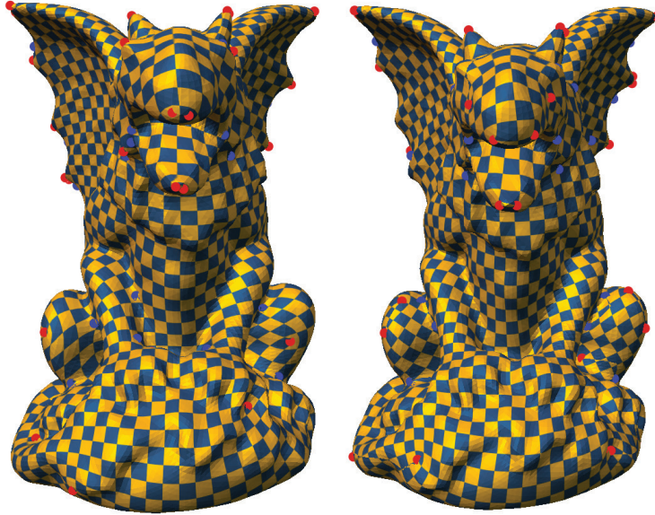
Figure 3.23: Comparison of extrinsic (left) and intrinsic (right) symmetry detection on an extrinsically symmetric model. There are small differences in cone placements but the global the field alignment is similar.
