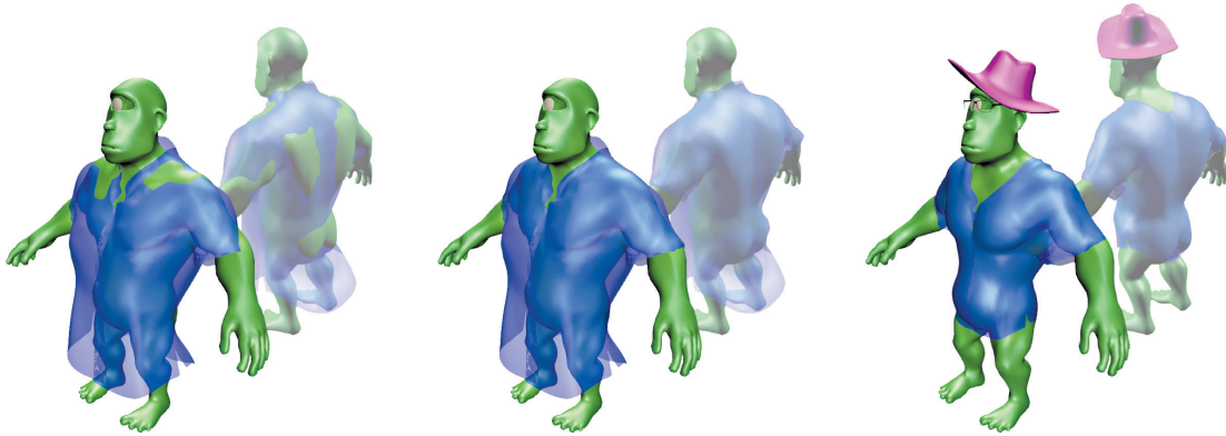
Figure 5.1: Interference-aware modeling greatly simplifies many complicated modeling tasks. We interactively fit the ogre with a shirt made for a human. We use our ability to fix existing intersections in a mesh and then “shrink-wrap” the shirt on the ogre, ensuring a perfect fit.
