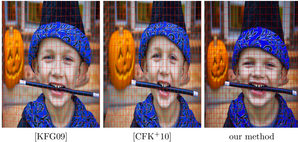
Figure 3.30: Excluding local rotations leads the retargeting deformation to be axis-aligned. The Child dataset, retargeted to half the width using recent state-of-the-art techniques and our method. Observe that although previous approaches do not explicitly enforce it, their deformations are effectively almost axis-aligned.
