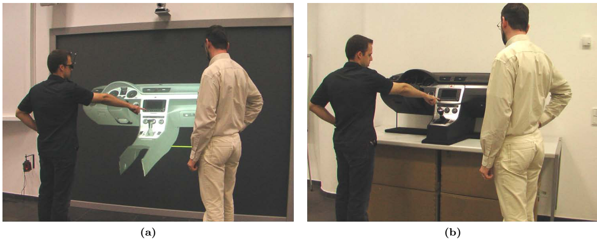
Figure 2.20: Multi-view virtual reality allows multiple users to interact with the virtual environment (a) as in real life (b). Image courtesy of Salzmann et al. [103]
