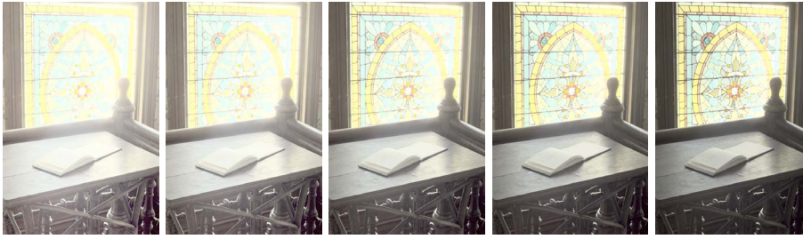
Figure 2.4: The effect of luminance adaptation over time, a simulation of the fast adaptation from a dark environment ( 10^{-4}\text{cd/m}^2 ) to the stained glass ( 17\text{cd/m}^2 ). Columns from left to right: t = 0.01\text{s} , t = 0.02\text{s} , t = 0.05\text{s} , t = 0.1\text{s} , t = 60\text{s} (fully adapted state).
