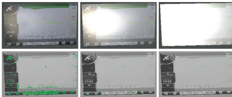
Figure 4.12: Visibility analysis of the displayed content subject to increasing level of reflections (250, 1250, 6250 \text{cd}/\text{m}^2 ).
