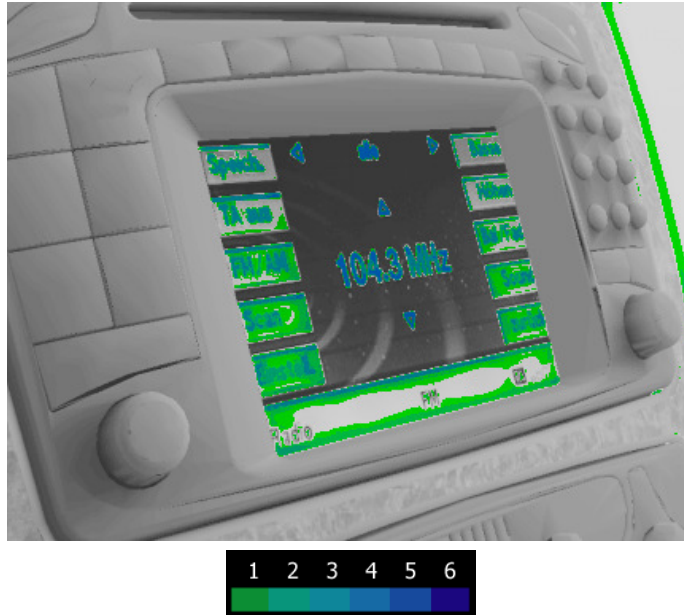
Figure 4.4: Visibility classes of the emission of a car display. Refer to Figure 4.1-right to see the original image.
