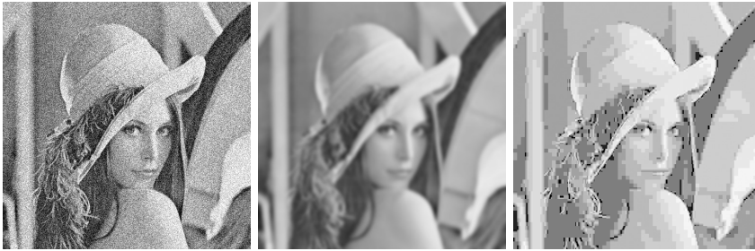
Figure 5.8: Sample images from our validation test set. We consider random pixel noise (left), gaussian blur (center) and JPEG compression (right) as distortion types.
