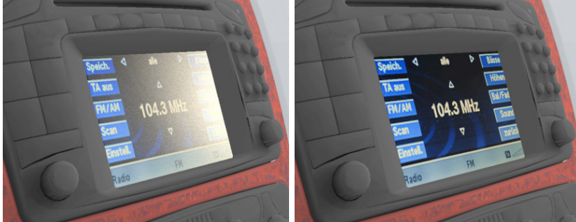
Figure 4.1: Images of a car display with and without reflections. Note that gamma corrected images should be converted to physical luminance before being processed by our method.
