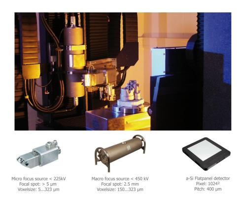
*Figure 1.1:* Dual source X-ray computed tomography device at Upper Austrian University of Applied Sciences - Wels Campus. Detail images of the main components: X-ray sources and detector (images are courtesy of Viscom, Comet and Perkin Elmer).
