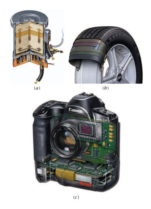
**Figure 2.10:** Illustrations based on different cut-away principles: (a) section view of an oil filter, (b) cut-away view with arbitrary and individual clipping geometries for various structures, and (c) ghosting illustration of a digital camera [31].
