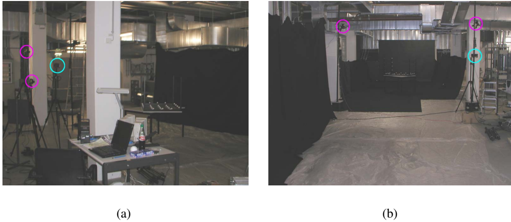
Figure 12.1: Ball acquisition setup. (a) A stereo pair of cameras (encircled in magenta) facing the black curtain on the right is capturing the ball’s initial flight parameters. The ball is illuminated by a stroboscope (cyan). (b) A second stereo pair of cameras (magenta) and a strobe light (cyan) facing towards the black carpet in the back are responsible for capturing the ball’s trajectory close to the “home base”.
