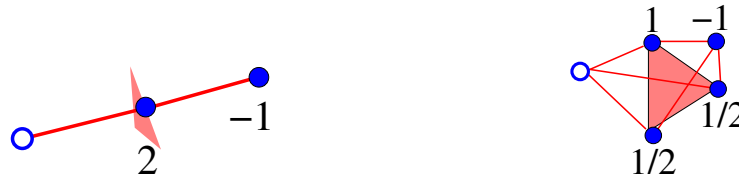
Figure 7.6: C^1 -smoothness conditions on a type-6 tetrahedral partition \Delta . The conditions are shown as the stencils of the two averaging rules which apply on \Delta , where the outlined Bernstein-Béziercoefficient is determined from the solid ones. The left stencil corresponds to the degenerate, univariate case (inter-cube and intra-pyramid, cf. Figure 7.5 (left)). The right stencil corresponds to the non-degenerate, general case (inter-pyramid, cf. Figure 7.5 (right)).
