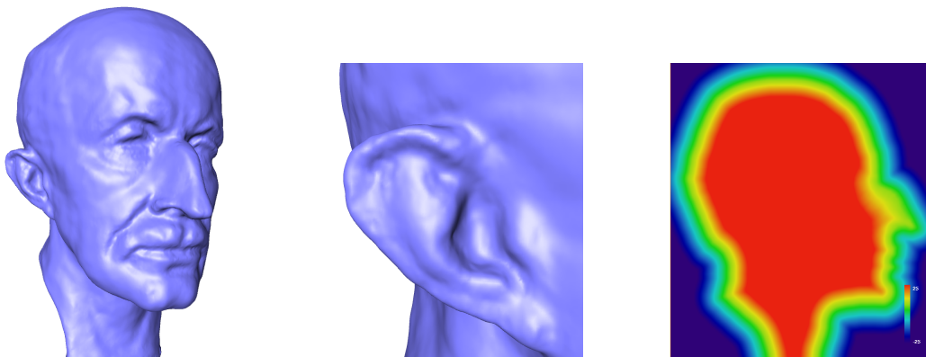
Figure 9.6: Visualization of the spline approximation s_{\text{planck}} for the Max-Planck data set. The domain is decomposed into 58 \times 97 \times 73 cubes. The left and center image show different views of the zero-set of the spline s_{\text{planck}} . The right image shows a slice through the approximative volume model s_{\text{planck}}(x, y, \text{const}) for signed distance values, where the distances are color coded.
