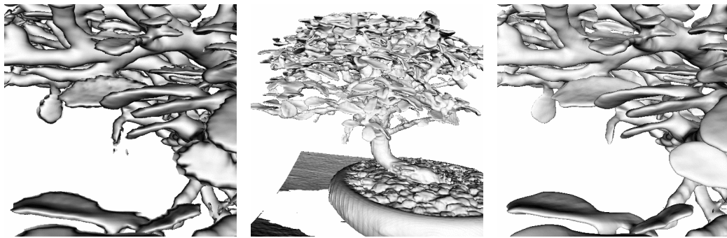
Figure 8.11: Isosurface of the bonsai data set (courtesy of Stefan Röttger, VIS, University of Stuttgart, Germany; 256^3 samples, isovalue 40). Trilinear (left) and our quadratic (center and right) reconstruction (7.1s and 9.1s, 3.1% relevant cubes).
