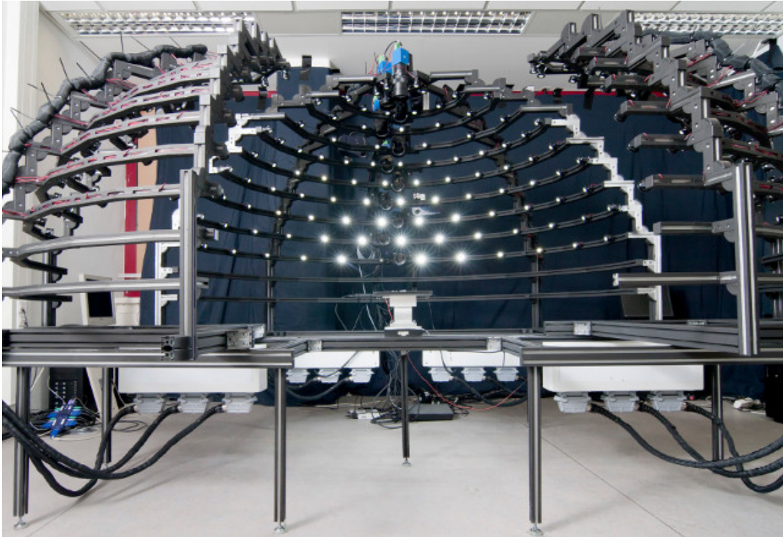
Figure 2.3: The Dome II, a BTf acquisition device developed by the University of Bonn [SSW + 14].
