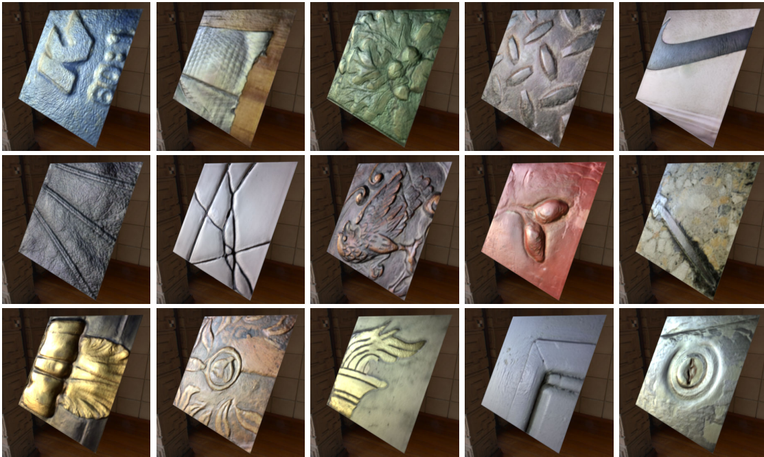
Figure 2.2: Examples of SVBRDFs rendered using a parametric model and a virtual environment.
