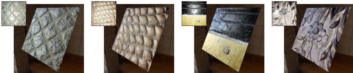
Figure 3.1: From a single flash photograph of a material sample (insets), our deep learning approach predicts a spatially-varying BRDF. See supplemental materials for animations with a moving light.
