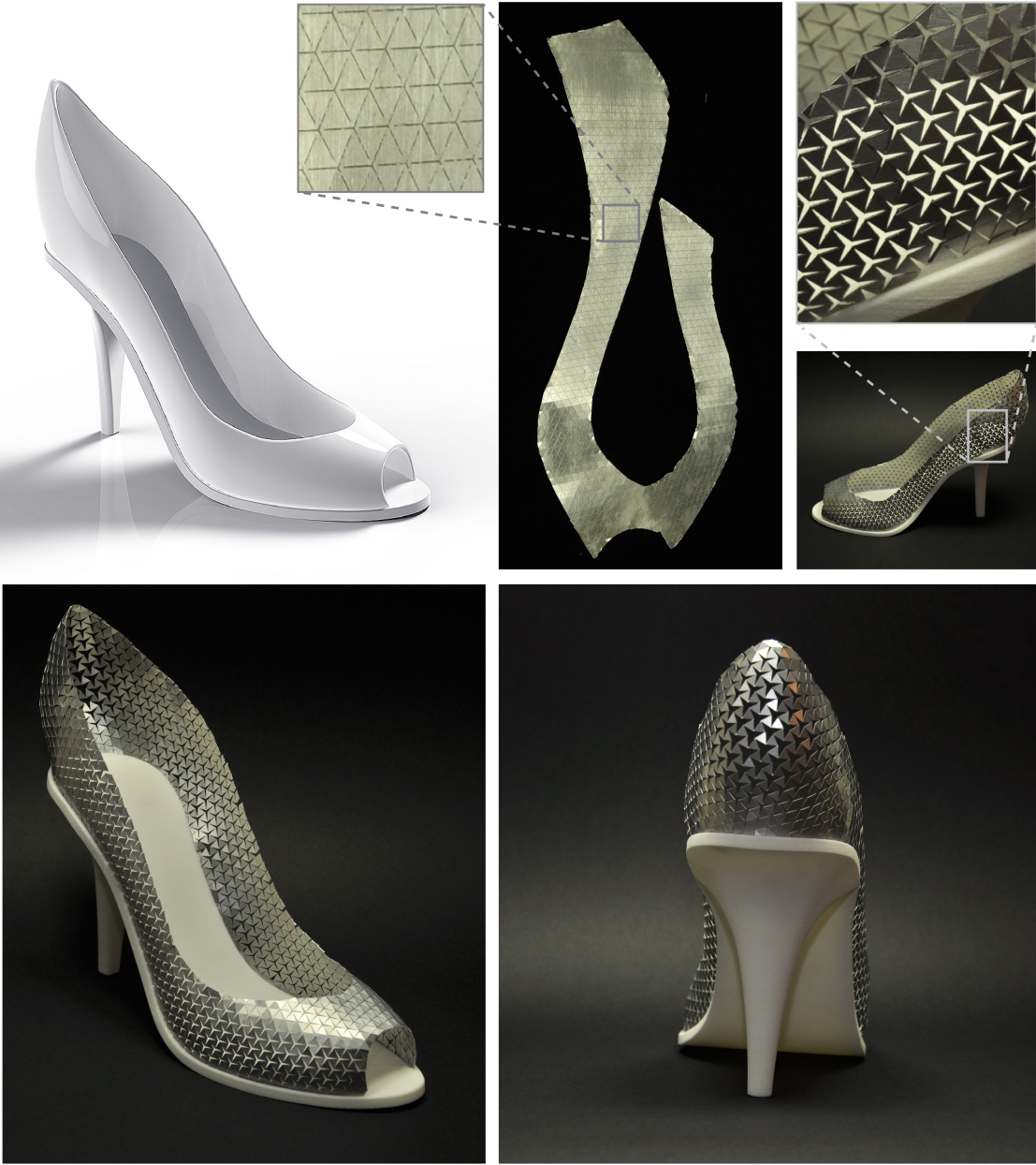
Figure 3.12 – The shoe model has been fabricated from a single piece of metallic material using our interactive rationalization method based on conformal geometry and global, non-linear optimization. Thanks to our global approach, the 2D layout of the material can be computed such that no discontinuities occur at the seam. The center zoom shows the region of the seam, where one row of triangles is doubled to allow for easy gluing along the boundaries. The base is 3D printed.
