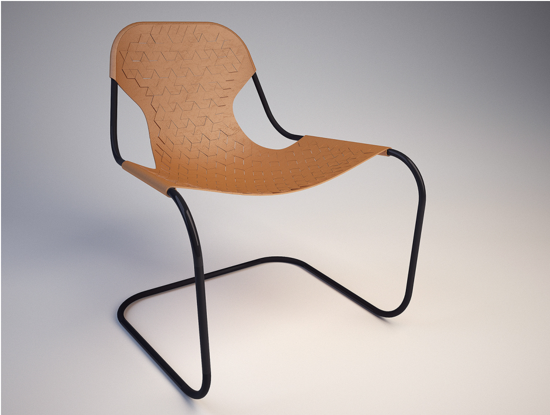
Figure 4.12 – Design study of a freeform chair realized using four layers of spatially graded auxetic material to fully cover the surface (see Section 4.4 for details).
