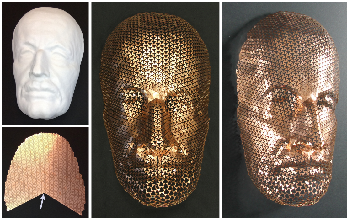
Figure 3.14 – Fabrication of the Max Planck model. Top left: 3D printed reference model used for geometric guidance; Bottom left: flat, undeformed perforated copper sheet. The purple arrow indicates the singular vertex located at the tip of the nose; Middle, Right: two photographs of the final model.
