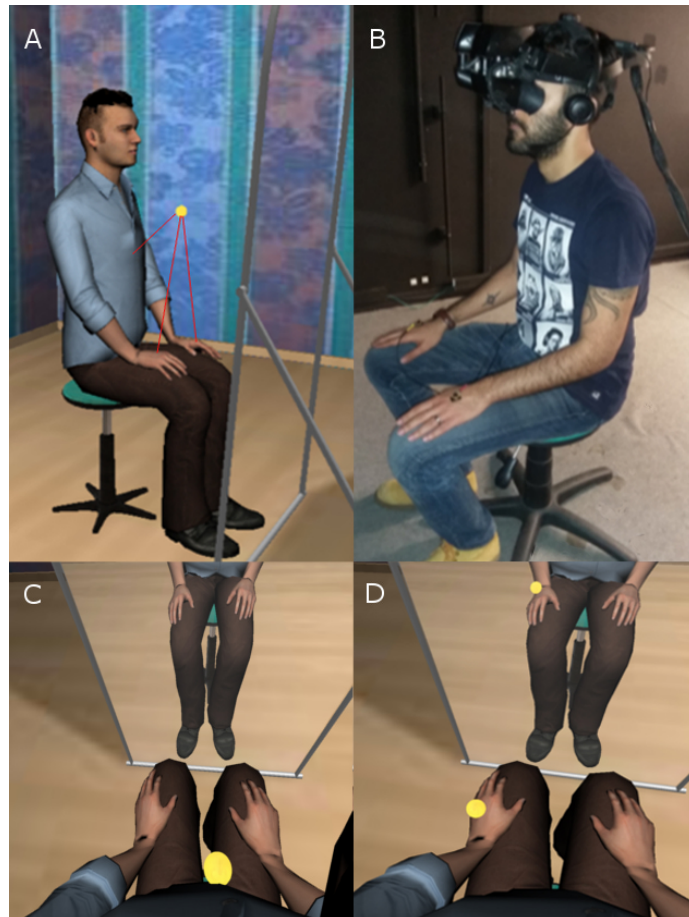
Figure 6.2: The experimental setup for Experiment 2. The body of the participant was substituted by a gender-matched virtual body, viewed from 1PP, onto which visuotactile stimulation was applied with the help of mechanical vibrators. The body could also be seen as reflected in a virtual mirror. (A) The collocated male VB showing in red lines the contact points of the virtual ball's trajectory with the virtual body counterparts. The tapping alternated among the three locations in random order. (B) Participant wore an HMD with a headset equipped with headphones and a microphone, and a set of mechanical vibrators attached to their hands and abdomen. (C) The male VB seen through the HMD from 1PP directly when looking toward it, and also in the virtual mirror when the virtual ball collided with the abdomen, and (D) with the left hand.
