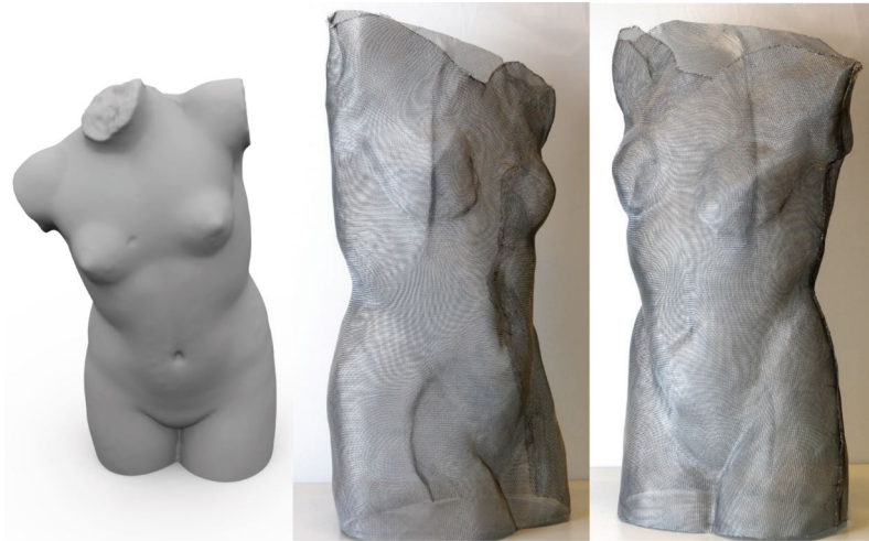
Figure 2.11: Fabricated wire mesh design [GSFD + 14] (center and right) of a 3D model (left).
