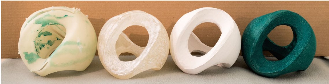
Figure 4.6: Sculpt model. Left to right: the flexible mold, the result of the cast using neutral resin, the cast with gypsum, and the cast with colored resin.
