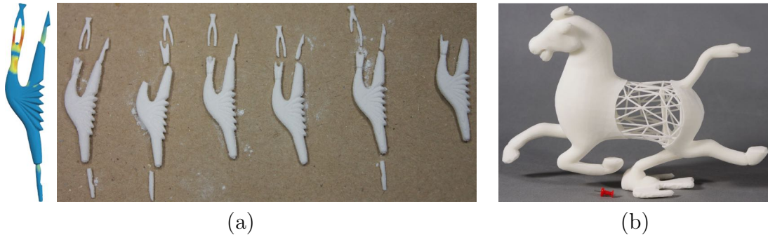
Figure 2.5: (a) A 3D model showing weak regions found with the method in [ZPZ13] and several 3D printed instances after a drop test; (b) a 3D printed model exposing the inner skin-frame structure generated with [WWY+13].
