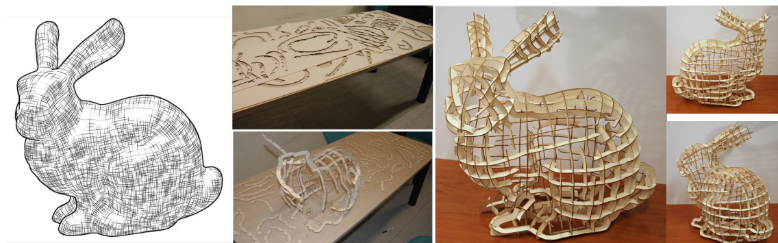
Figure 3.1: Given a 3D shape with a smooth cross-field, we generate a set of planar slices that can be interlocked in a self-supporting structure.
