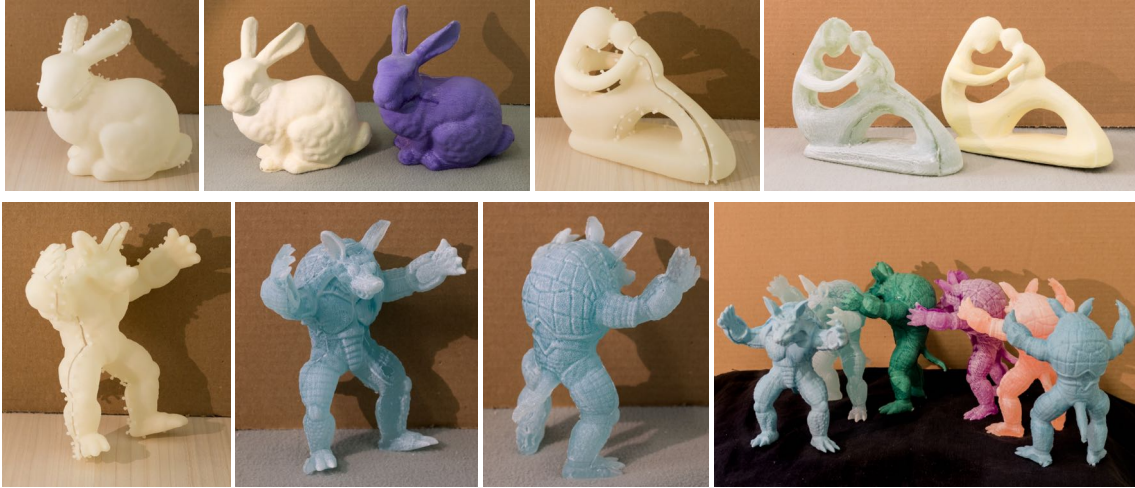
Figure 4.22: Molds and casts obtained for the bunny, the fertility, and the armadillo models.
