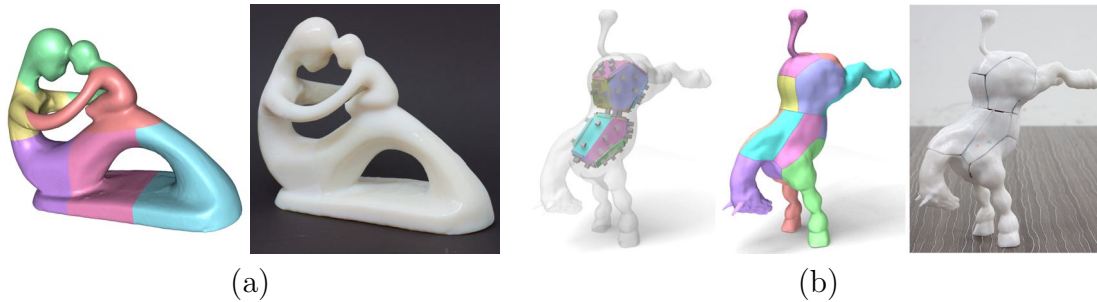
Figure 2.2: (a) A model partitioned by Chopper [LBRM12], then 3D-printed and assembled; (b) an assembled horse model produced with CofiFab [SDW + 16].
