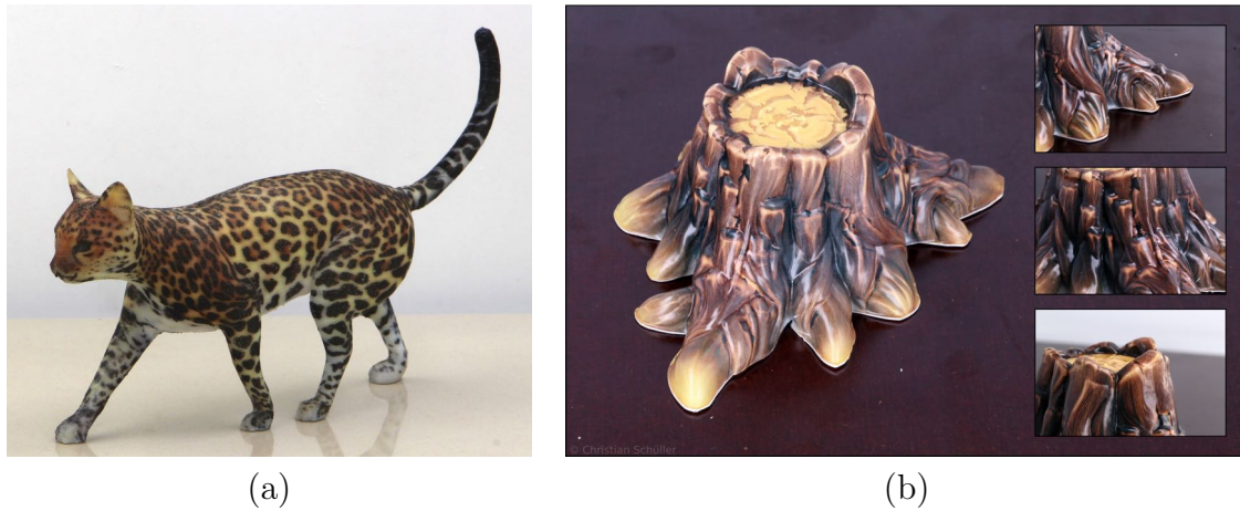
Figure 2.4: (a) 3D printed model colored with the hydrographic printing technique in [ZYZZ15]; (b) colored miniature stomp obtained with the thermoforming method in [SPG + 16].
