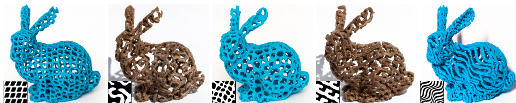
Figure 4.1 – Our by-example pattern synthesis algorithm produces structurally sound patterns along the surface of an object, resembling the input exemplar. The reinforcements are integrated within the pattern, by a joint optimization of appearance and structural properties. Top: The Stanford bunny with a variety of synthesized patterns. Bottom: Example patterns. These objects are printed in ABS plastic on low-cost filament printers, using a dense support. The patterns are fully connected and survived the cleaning process thanks to their reinforced structure. Yet, the reinforcements are inconspicuous as they seamlessly blend within the appearance.
