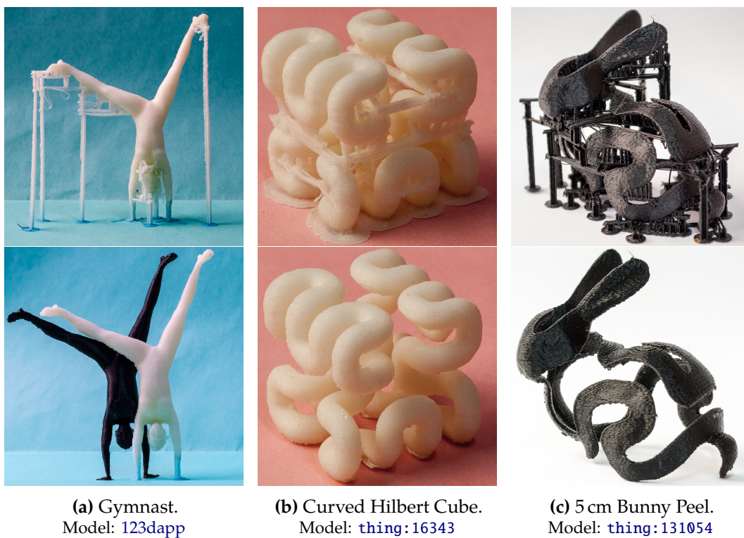
Figure 3.17 – Models printed with our technique, with their scaffoldings (top) and cleaned models (bottom).
