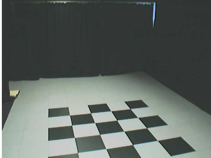
Figure 3.3: Camera calibration pattern on the stage floor, viewed from one camera.
