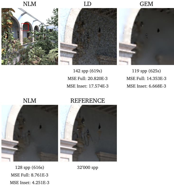
Figure 7.17: Renderings of the “sanmiguel” scene using a variety of methods. Non-filtered uniform low-discrepancy sampling (LD); our previous method described in Chapter 6 (GEM); our method with adaptive low-discrepancy sampling (NLM). All results for a given scene have an equal rendering time, to account for each method overhead. We use the default filtering window size, r = 10 . The MSE values are listed under each image and the corresponding SSIM values are given in Table 7.1.
