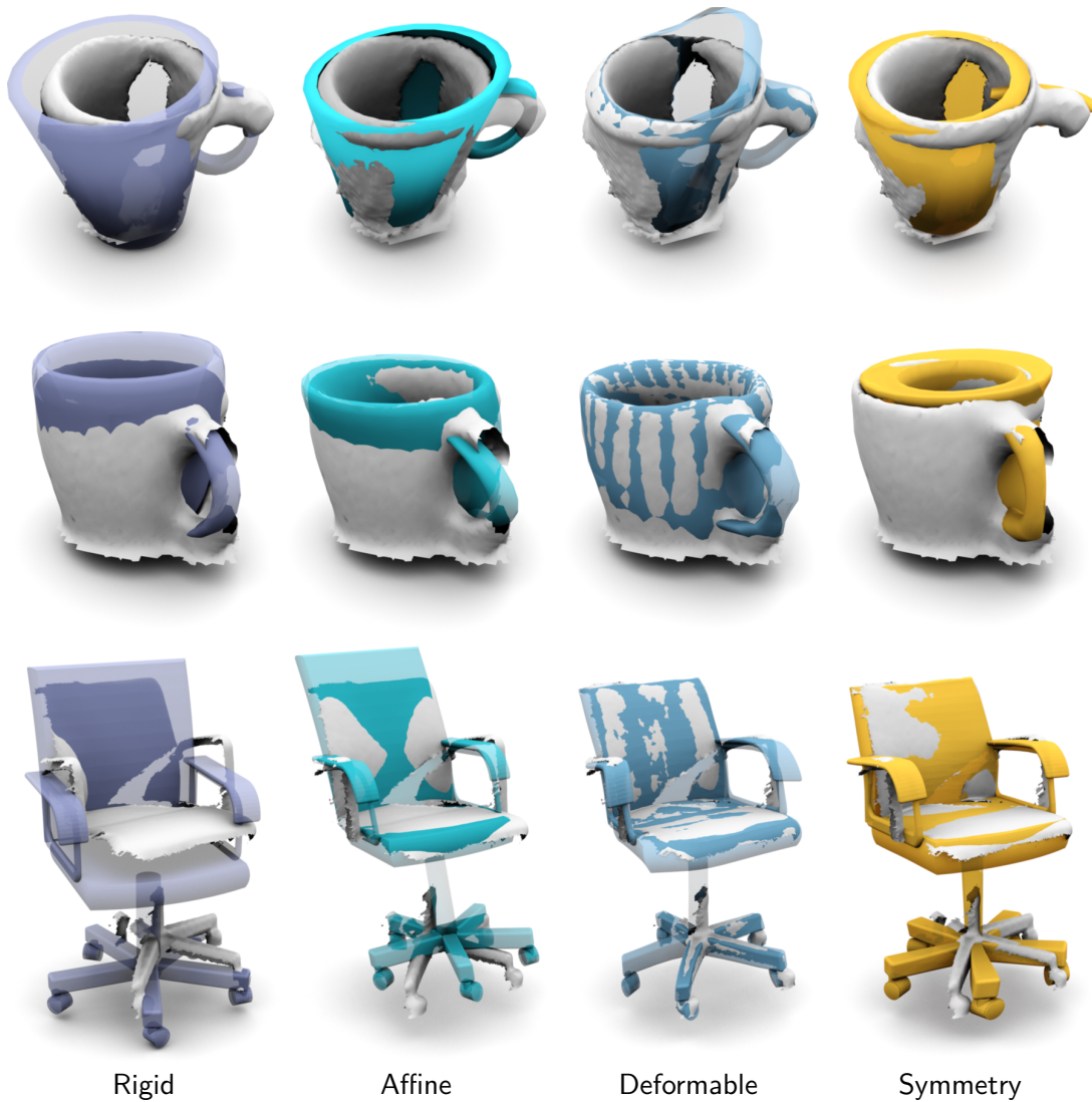
Figure 6.8: Overlays of the deformed models and the corresponding target shapes. From top to bottom: cone-shaped cup; rounded cup, office chair (single-view). In complex cases where no tight template is available, only the deformable ICP variants can match the data closely. Symmetry is able to preserve the structure better, as has already been shown in previous figures.
