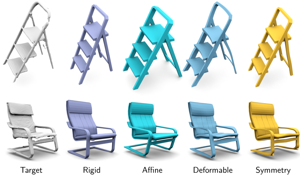
Figure 6.16: Full scan of a stepladder (top) and of the armchair from Figure 6.5 with a different template model (bottom). The Symmetry results are very close to the template model and consequently not a good fit for the target shapes. This is due to spurious symmetries in the template models: in combination with the continuous symmetry constraints, deformation is prevented.
