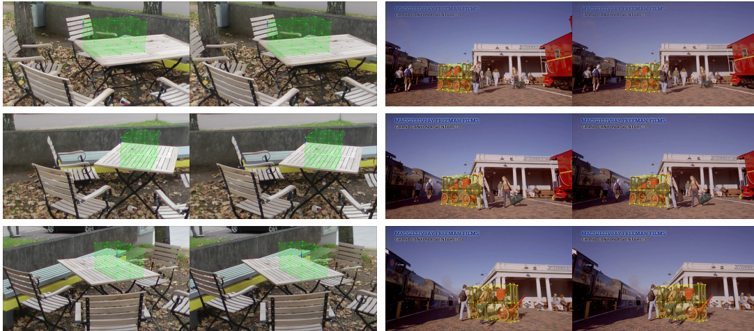
Figure 3.7: Real-world experiments: The frames on the left depict garden furniture and were recorded using a consumer HD camcorder with a 3D conversion lens. The frames on the right depict a scene at a train station and were recorded using professional equipment. Both sequences were augmented by a cuboid to demonstrate the quality of the estimated camera parameters.
