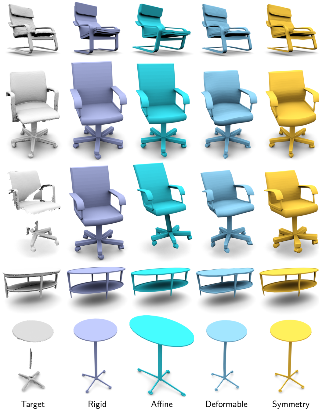
Figure 6.5: Results of different ICP variants. From top to bottom: Armchair (full scan); office chair (full scan); the same office chair (single-view); oval table (full scan); bar table (single-view).
