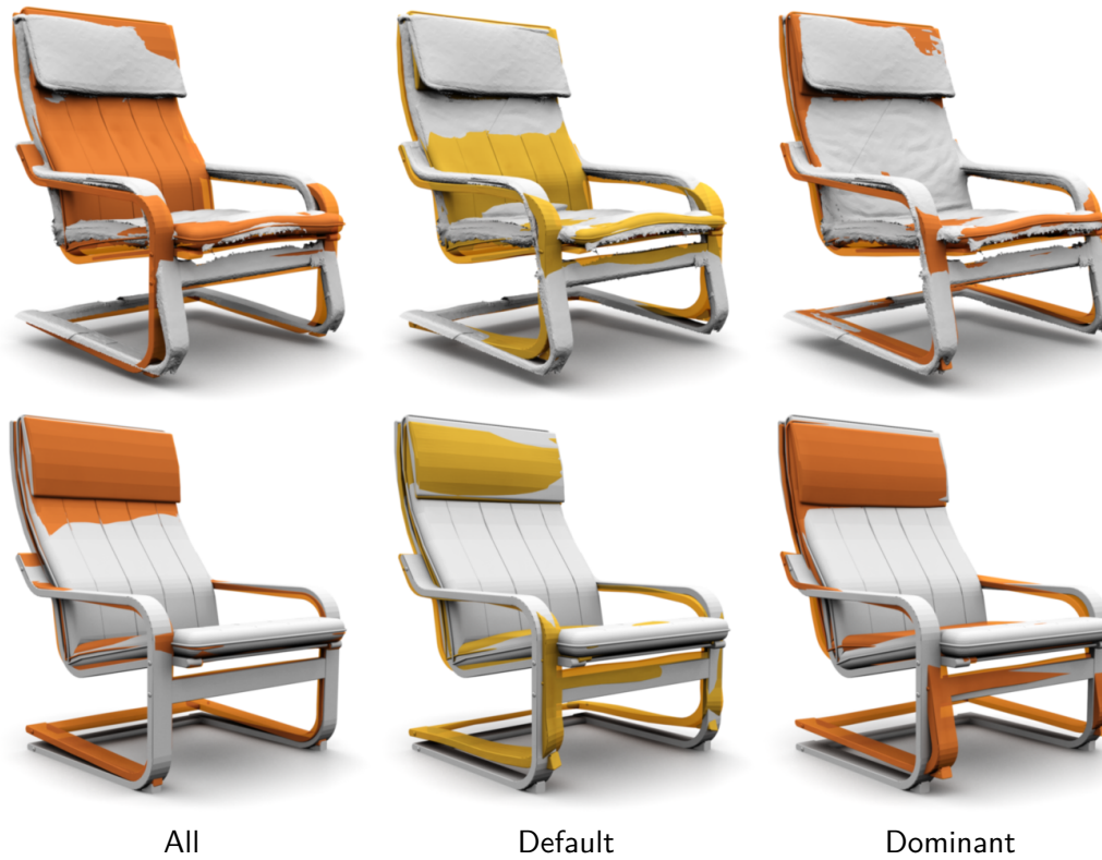
Figure 6.17: Overlays of Symmetry over the corresponding target shape (top) and the template model (bottom). The overlays are shown for different sets of symmetry constraints: For Dominant , only the most significant symmetry (a global reflective symmetry in this case) is kept. The deformed model largely deviates from the original model, but is almost a perfect match for the target shape. Default represents the set of symmetry constraints retained during normal processing. The additional symmetries compared to Dominant start to restrict the deformation, preventing the frame of the chair to be represented faithfully. All shows the result for all detected symmetry constraints enforced. There is almost no deformation due to interlocking constraints; only the bottom of the frame is able to extend upward.
