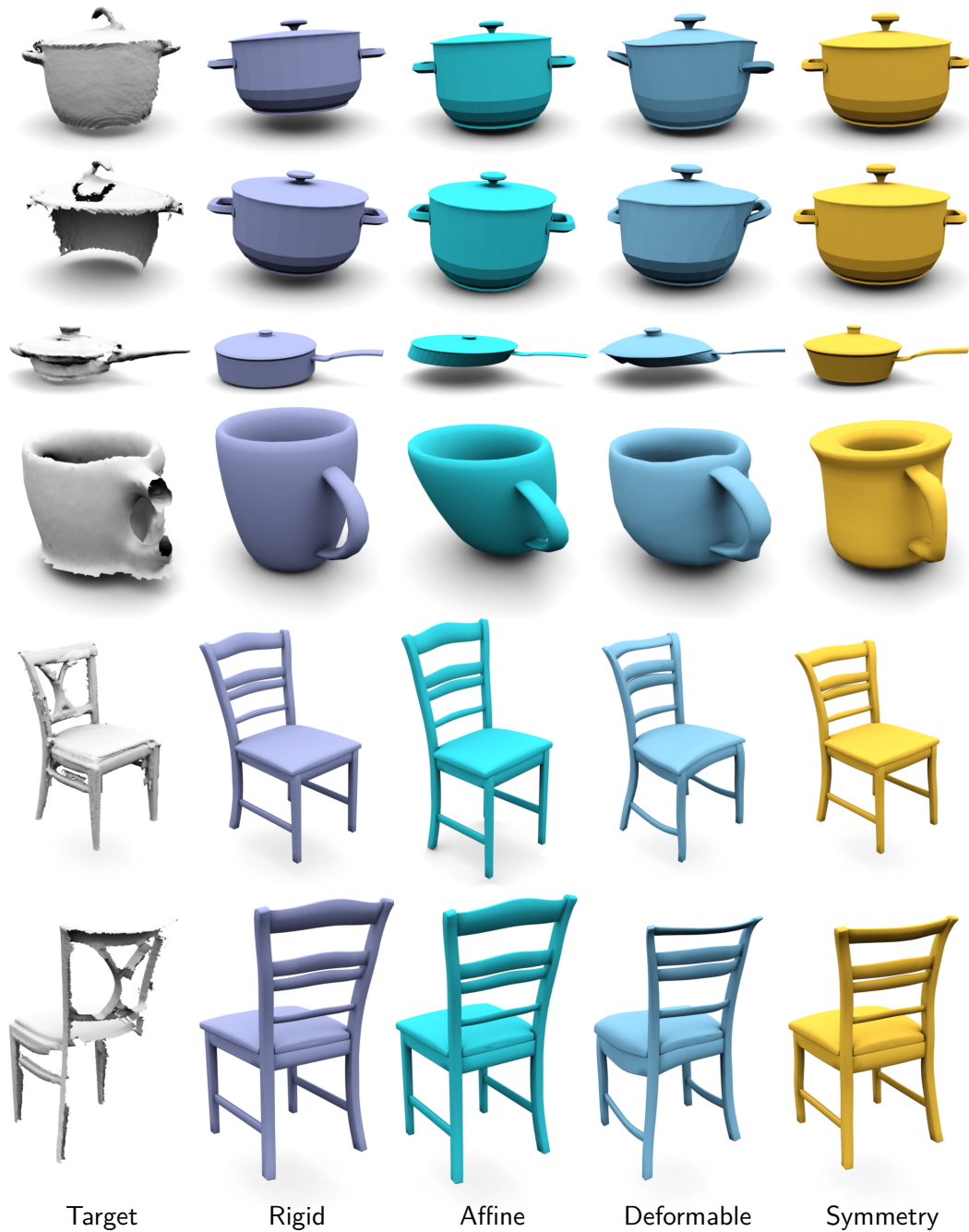
Figure 6.4: Results of different ICP variants. From top to bottom: Cooking pot (single-view, front); the same pot (single-view, back); frying pan (single-view); rounded cup (single-view); chair (full scan); the same chair (single-view).
