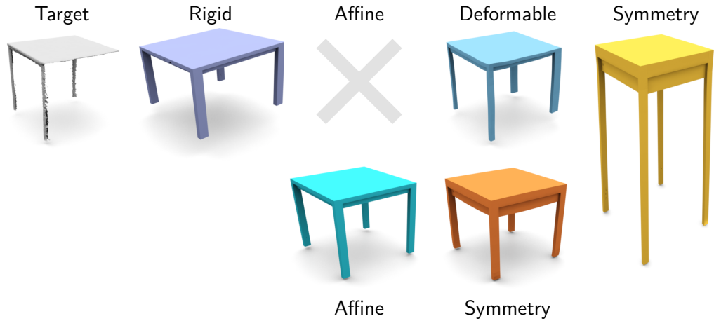
Figure 6.18: Partial scan of a square table. The elongation of the table in the Symmetry result is caused by the failure of the ICP algorithm to find a stable set of correspondences due to the constraints on the deformation field. Affine completely diverges for the same reason. For the results in the bottom row, a single handle constraint has been attached to a table leg manually.
