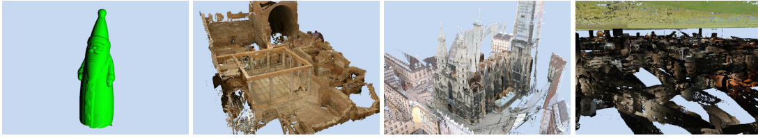
Figure 3.20: The scans used for benchmarking the build-up algorithm and the editing operations. Left: Santa Claus model, consisting of about 16M points. It was scanned with a scan-arm. Center left: Model of the “Hanghaus” in Ephesos, consisting of about 15M points. Center right: The Stephansdom in Vienna, consisting of 193 single scans and about 460M points. Right: A view of the subterranean Domitilla catacomb in Rome, hovering below the turf. This model consists of 1828 single scans and about 1.92 Billion points.
