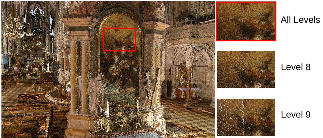
Figure 3.16: The points of the different levels are blended to make a closed surface of the point model. In the closeup, points from hierarchy level 8 and 9 are shown. All levels combined result in the closed surface for the point model.
