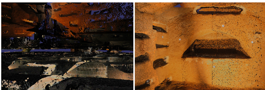
Figure 4.2: In the left image, the viewpoint is hovering between the 1st and 2nd floor of the catacomb, showing the detailed scanning of the galleries. The right image shows a cubiculum from the inside. The registration markers are clearly visible.
