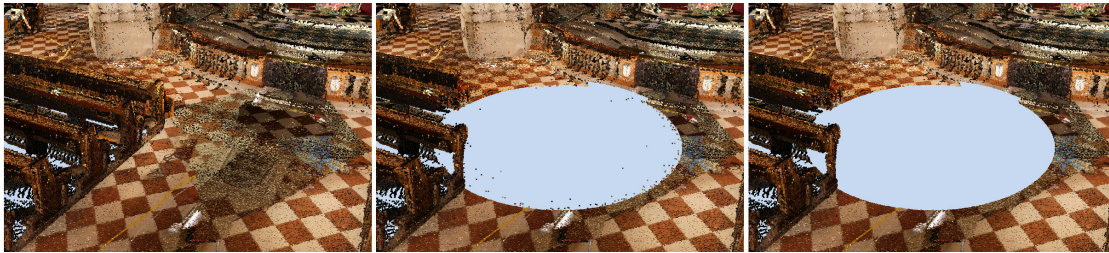
Figure 3.19: From the original point cloud (left image) a spherical volume is deleted. The center image shows the artifacts that remain when the interior nodes are not updated after deleting points. In the right image, the points in the interior nodes have been updated according to the deleted volume.
