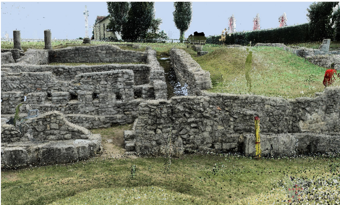
Figure 4.9: In the upper image, the points of the Amphitheater 1 model are rendered as square splats, and each splat is rendered with one color. The single stones of the wall are not clearly visible due to color noise and overlapping splats. In the bottom image, the points are rendered as Gaussian splats. The single stones of the wall are clearly visible due to the reduced color noise and blending of overlapping splats.
