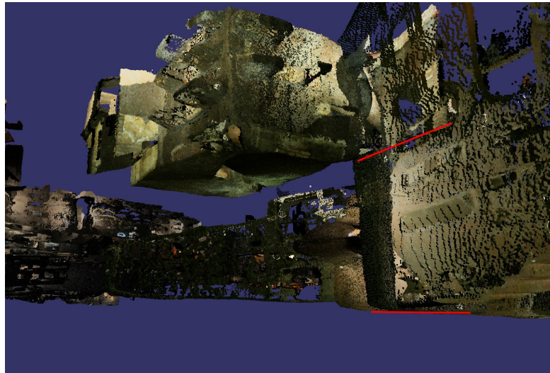
Figure 4.3: This cubiculum in the region “Flavi Aureli” cannot be reached at-grade. The red lines denote the different height levels of the floor (a difference of more than 2 meters) and were later added to the image for visualization.
