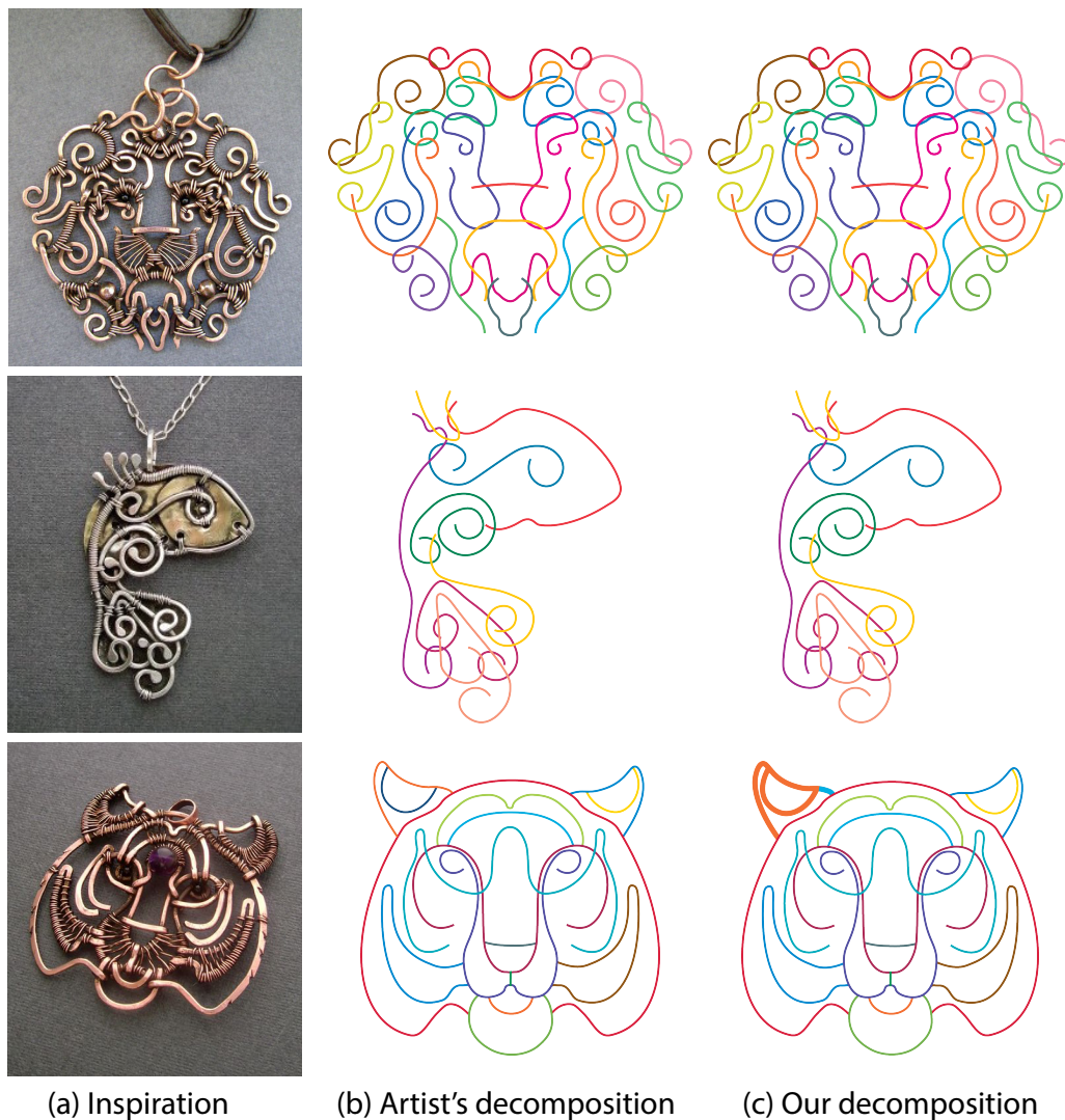
Figure 3.5: We use existing jewelry (a) as inspiration to test our algorithm. . Our solution (c) closely matches the Artist's original decomposition (b). The decompositions are identical for the lion and the fish, while the left ear of the tiger results in a slightly different configuration than the original, although with the same number of wires.
