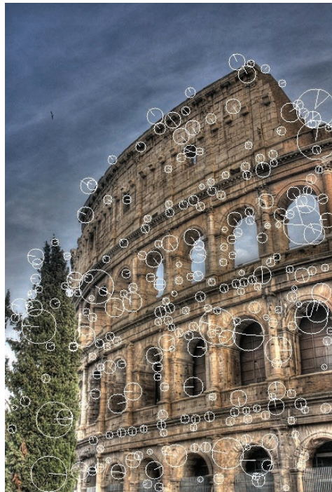
Figure 2.12: Feature detection using DoG. Each circle represents the scale and orientation of a feature.
