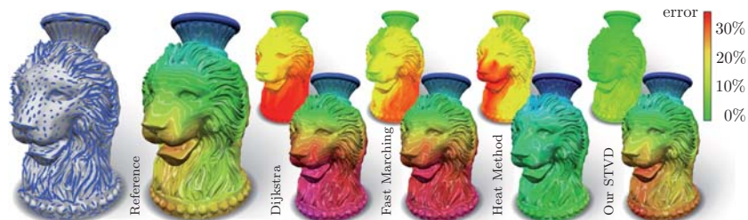
Figure 9.1.: Visualization of a geodesic distance field with respect to an anisotropic metric (shown by tensor ellipses on the left; field source on top). Next to a reference solution, we show the results and approximation errors of various adapted known algorithms applied for the distance computation. Our novel Short-Term Vector Dijkstra on the far right shows the best results.
