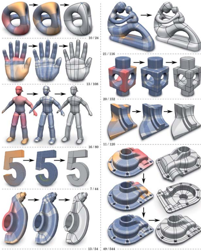
Figure 8.5: Quad layouts designed with our interactive method. Shown are intermediate design stages with dual strips and region coloring, followed by the final quad layout. Next to each layout the number of dual strips and the (typically much larger) number of primal layout arcs is specified.
