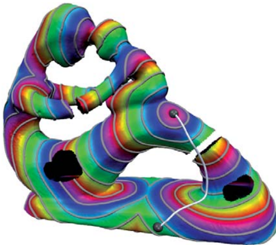
Figure 10.1.: An intrinsic distance field and a geodesic path computed on an imperfect mesh in a defect-tolerant way.
