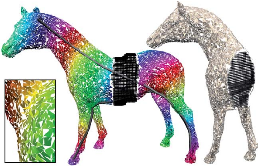
Figure 10.7.: Inconsistent polygon soup with a slice cut out. Dilated cells that survived erosion, a distance field, and two geodesic paths are visualized. Increasing the gap width at some point leads to the morphological operators closing the two holes instead of bridging the gap, as depicted on the right.
