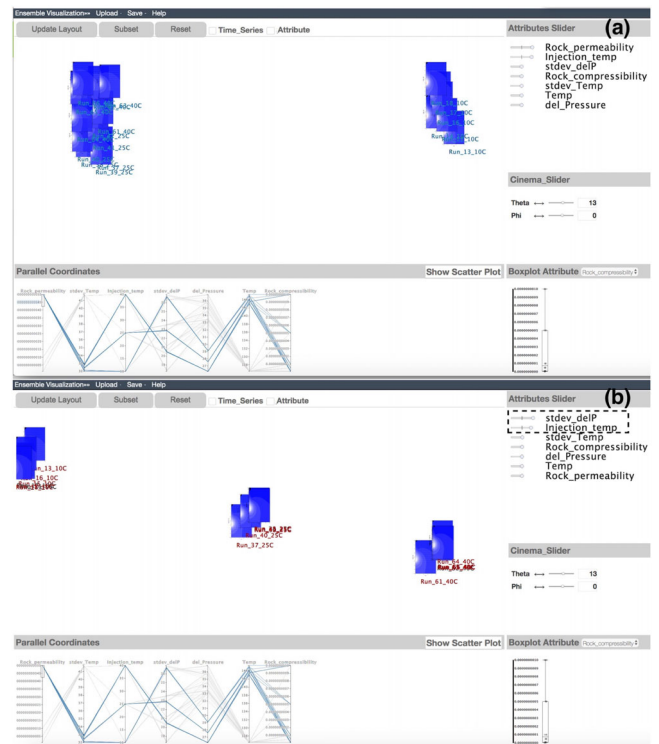
Figure 11: (a) Scientists investigate what differentiates the highest fluid pressure build-up runs by dragging and clustering runs based on deepness level, then performing OLI. (b) After clicking 'Update Layout', they gain an insight that pressure magnitude of these deep runs is governed by the temperature of injection fluid.
