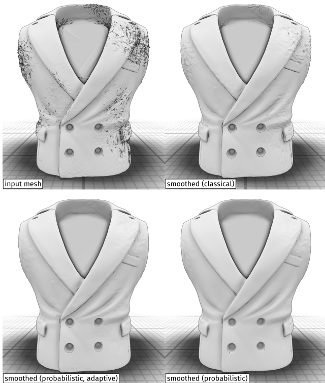
Figure 4: Quadric-based mesh smoothing. The input mesh shows strongly spatially varying noise. Classical quadrics (top right) preserve features and smooth over some noise but are unable to suppress stronger noise completely. With probabilistic triangle quadrics and a high value for \Sigma (bottom right), the noise can be almost eliminated but smaller features are smoothed over. Using heuristics (such as the angle defect) to estimate the local noise level, adaptively changing \Sigma smooths over the noise while preserving features (bottom left). Model from [ZJ16].
