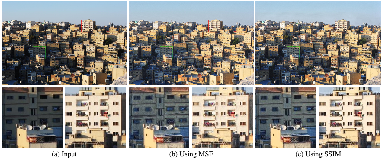
Figure 2: Comparison with using SSIM instead of MSE for the artifact suppression loss.
