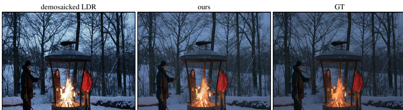
Figure 7: An example of challenging simulated scene with a very large dynamic range (over 30 stops) zoom in for better view. Left: demaicked LDR image for illustration purpose note the complete saturation in the fire region, Middle: tone-mapped HDR images for our results note the artifact in the saturated region. right: tone-mapped ground truth HDR image.
