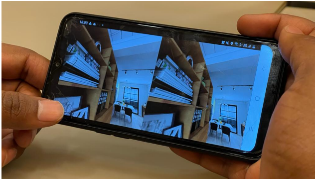
Figure 9: SPIDER-mobile application. The stereoscopic renderer is deployed on Android platform, and the indoor scene can be interactively explored through touch interface or by using IMU sensors for simulating head movements and ready for VR headset like Google Cardboards.
