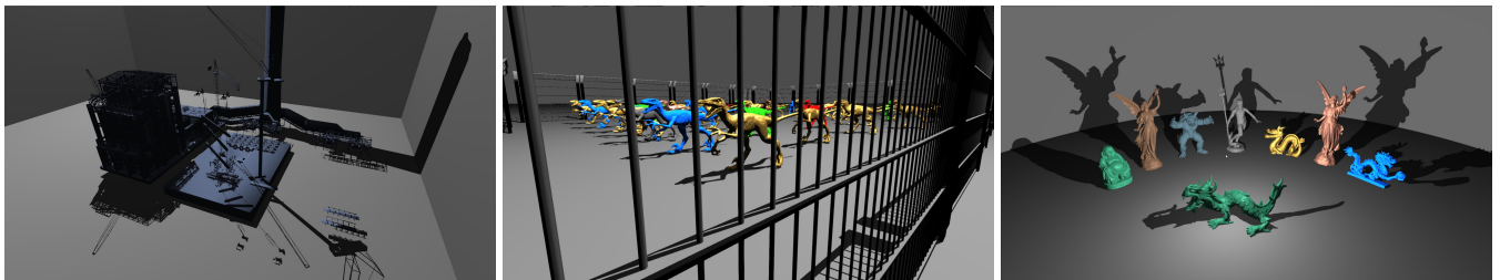
Figure 1: Three scenes rendered using our shadow algorithm. Left: Powerplant (12.7M triangles) 20ms. Middle : RaptorPark (30M triangles) 17ms. Right: ManyModels (73.8M triangles) 28ms.
