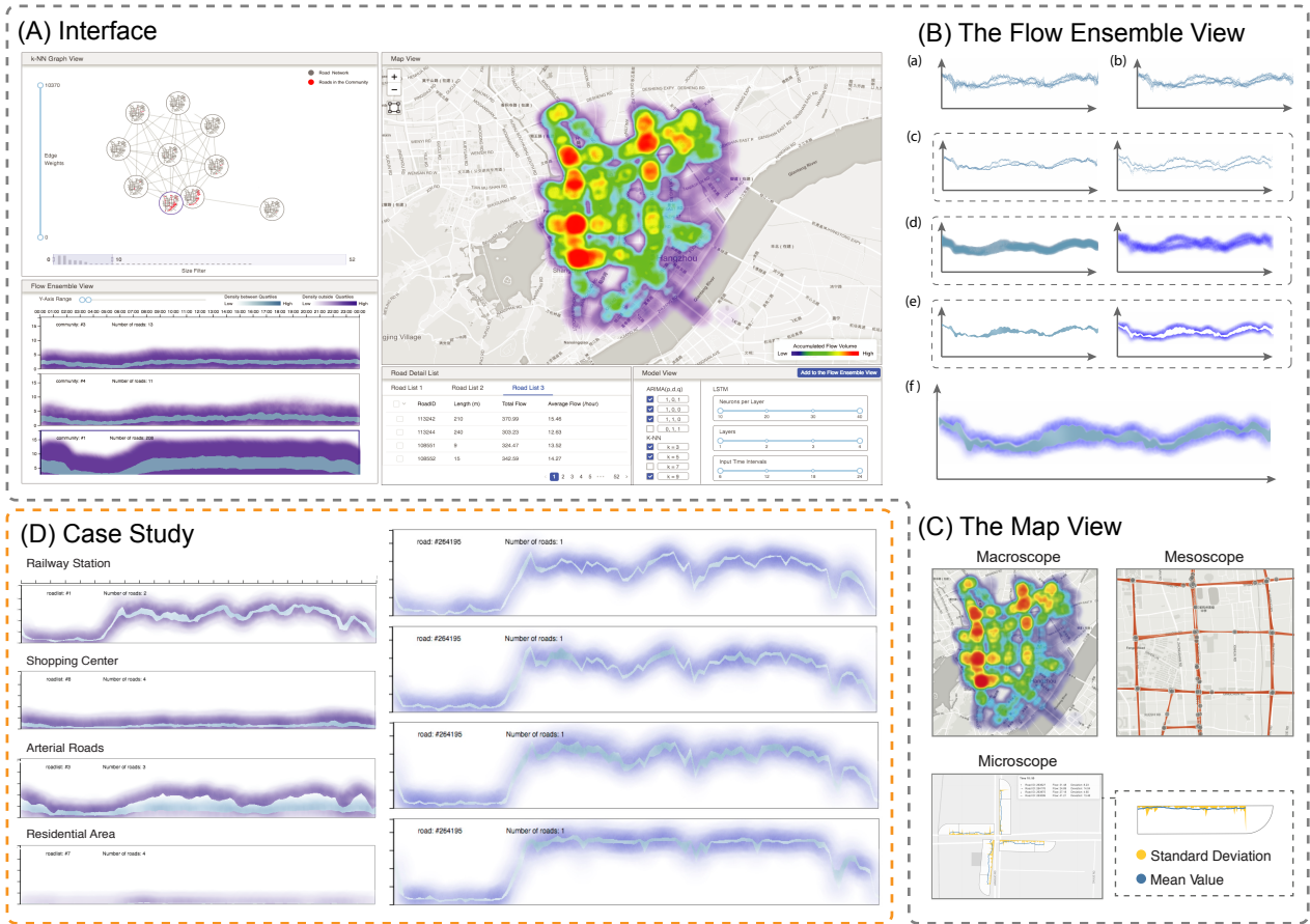
Figure 1: (A) The visual interface of our system. (B) An illustration of the flow ensemble view. (C) Visual design of the multi-level temporal map view. (D) The flow ensemble views (Left) of four functional regions selected in the case study, and (Right) four different parameter configurations.
