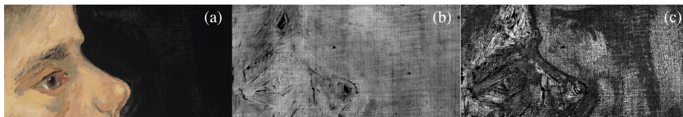
Figure 1: Scans of part of a painting, showing (a) color, (b) height map and (c) gloss map, describing the appearance of the surface
