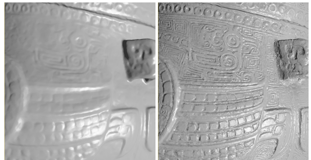
Figure 4: The results of the surface normal estimation method for the you dataset. Left: the input geometry with per-vertex normals. Right: the same geometry rendered with the computed normal map. See Figure 1 for final results.
