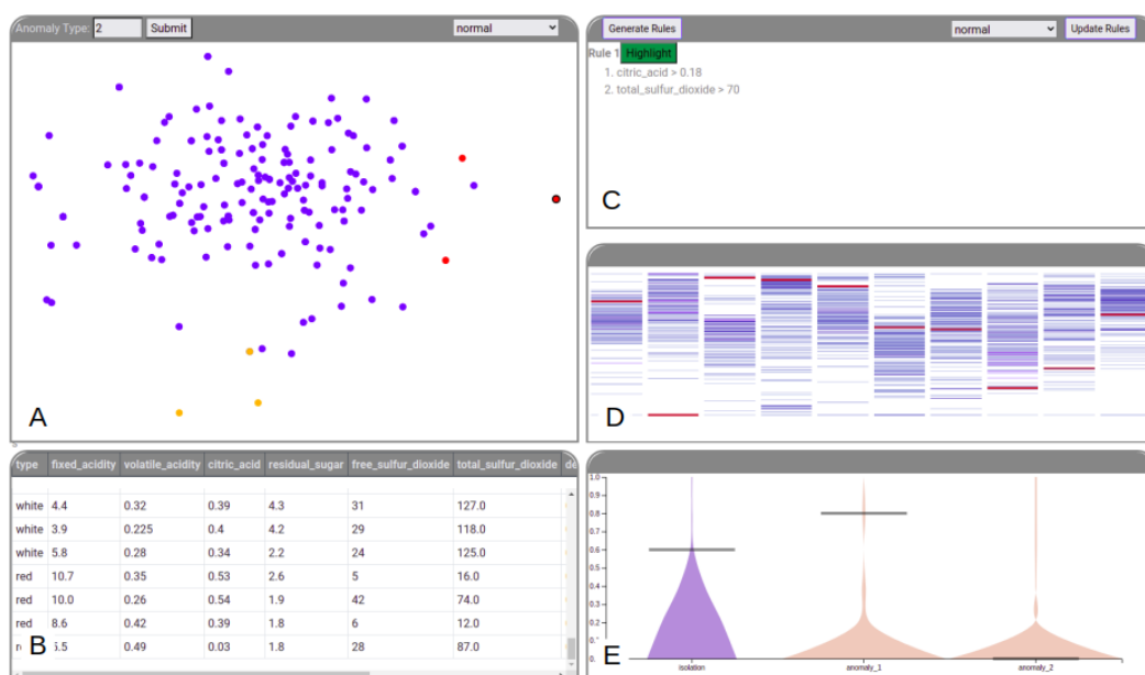
Figure 1: RISSAD prototype: A) scatterplot, B) data table, C) descriptive rules, D) data distributions, and E) isolation and similarity scores.
