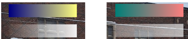
Figure 1: LEFT: The top colourmap is a non-isoluminant one. The bottom colourmap is created by converting the top colourmap’s luminance to opacity to simulate the visibility on an additive HWD. More opacity means better visibility. We observe that low-value colours are very transparent. A photo of a Masonic temple was used to illuminate the effect. RIGHT: The top colourmap is a more isoluminant colourmap used in the study. We can see that the visibility is higher for the lower values (bottom).
