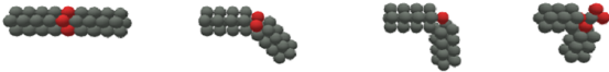
Figure 3: The described joint implementations. From left to right: stiff joint, hinge joint, ball and socket joint and universal joint.
