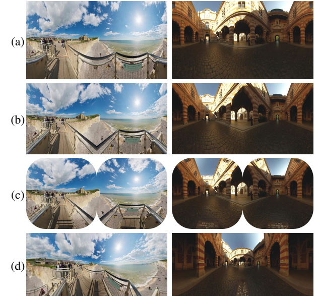
Figure 3: Full spherical panorama visualizations. (a) The cylindrical projection. (b) The Pannini projection. (c) The swung-to-plane projection. (d) Our swung-to-cylinder projection.
