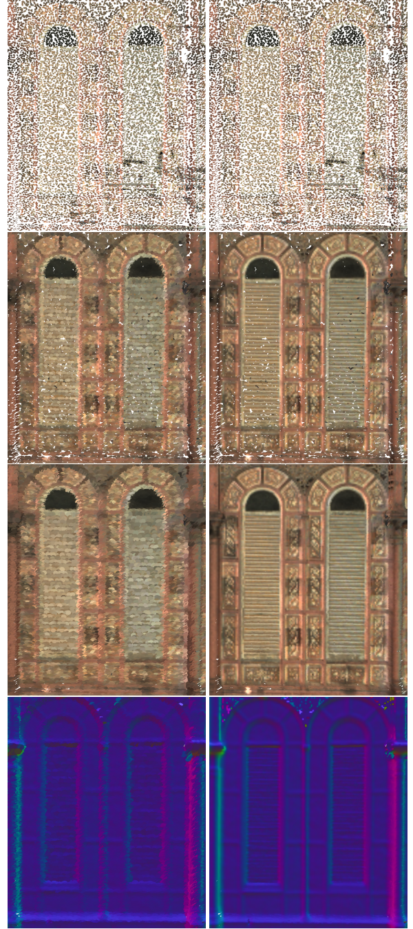
Figure 2: Renders of a point cloud using simple splats (left) and our method (right). We are using a tenth of the original points, increasing the splatting radius to fill the holes. Regular splats appear completely flat and the high frequency detail is lost. Our method assigns a texture coordinate to each fragment and thus we are able to reproduce the high frequency features for both color (rows 1 through 3) and normal data.
