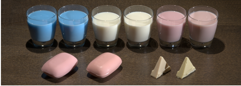
Figure 3.2: A side by side comparison of real translucent materials (right) next to their silicone replicas (left) fabricated using our method.
