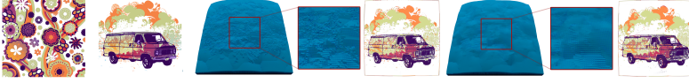
Figure 4.4: Source/target images (left pair) are mapped with a source-optimized lens without (middle set) and with (right set) simulated annealing. Simulated results are indistinguishable but the lens generated with simulated annealing is smoother and manufacturable. The lens ( 128 \times 128 facets with 11 \times 11 micro-facets) is designed to be placed at 10 cm from the source and 40 cm from the viewer.
