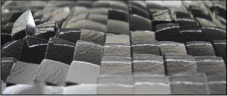
Figure 4.13: A photographic zoom-in of one of our 3D printed steganographic lenses. Notice the easily visible z layers deposited by the printer and the semi-transparent nature of the printing material.
