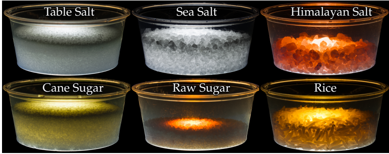
Figure 5.3: A selection of real granular materials illuminated from underneath with a cell phone’s flash light to reveal their translucency. Granular materials can exhibit long-range light transport that still retains complex small-scale structure. Each HDR capture was individually tone-mapped for display.
