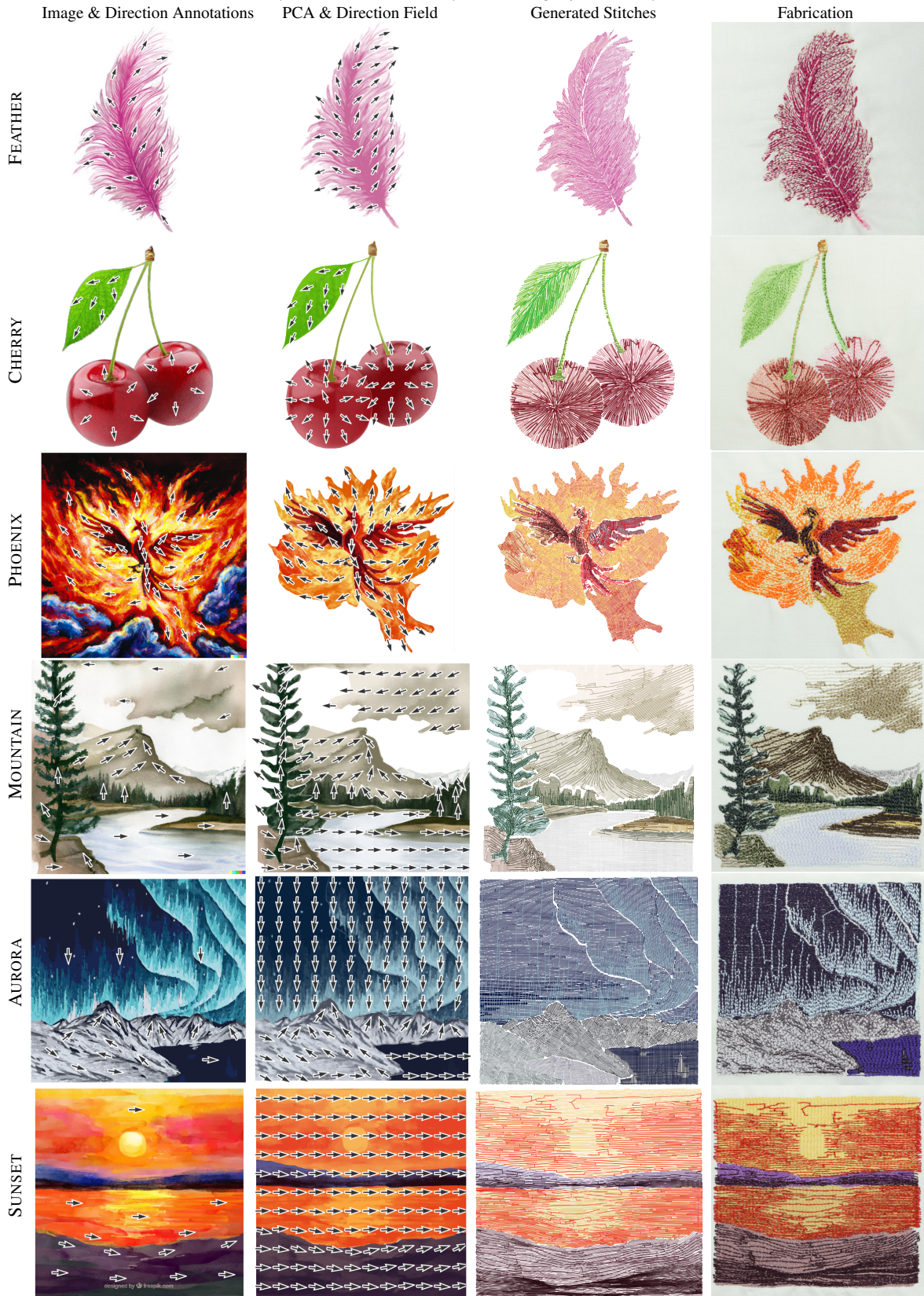
Figure 14: Different embroidery patterns produced by our method. We show the original image with direction annotation, the segmented PCA image superposed by the direction field, the generated stitching pattern, and the photos of the patterns sewed by an embroidery machine.
