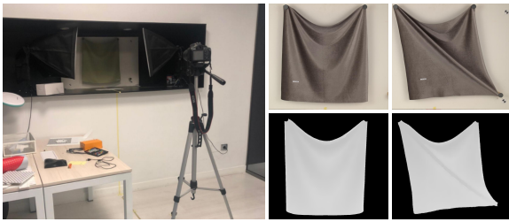
Figure 2: Capture setup, RGB (top), and depth (bottom) images for hanging (left) and stretch (right) scenes in rest position. Each scene conveys a different mechanical appearance of the fabric: hanging exhibits the overall drape; stretch exhibits an extra diagonal tension, which is key to understand the stretching properties.
