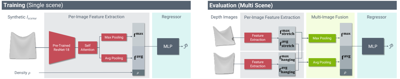
Figure 6: Diagram of our training and evaluation pipelines. For training , we use a single image of the material, along with its density. The image is processed by our Feature Extractor, followed by an MLP, which computes the parameter estimation \hat{P} . For evaluation , we process each available image with our trained feature extractor and use a fusion operator before feeding it to the trained regressor. We use the same Feature Extractor and MLP for both scenes.
