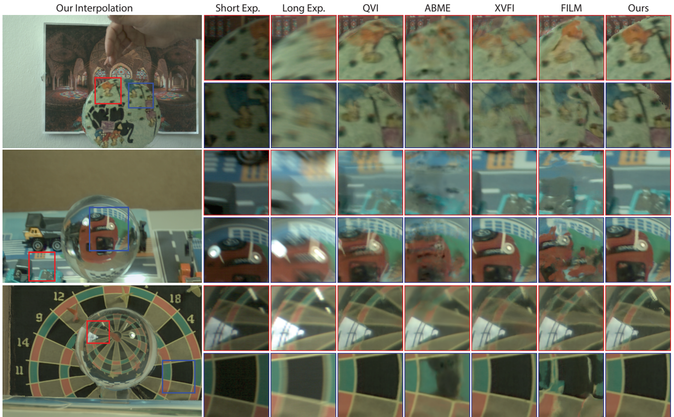
Figure 8: The visual comparisons of our interpolation results for three scenes captured using our camera with a dual-exposure sensor: Our method is able to correctly interpolate the frames in the scenes with the challenging cases of a rolling disc (the upper scene), a rotary camera motion (the middle scene), and a moving object behind a refractive object (the bottom scene).
