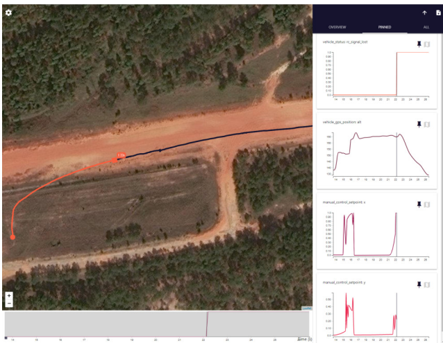
Figure 7: Flight log from a UAV that experienced a malfunction visualized with DATA COMETS. UAV lost radio control (RC) connection and entered a fail safe landing mode. Using the pin tab to display the relevant data we can see the exact moment rc was lost and how other attributes were effected by this. Encoding the RC connection attribute onto the flight path shows exactly where the malfunction happened geospatially.
