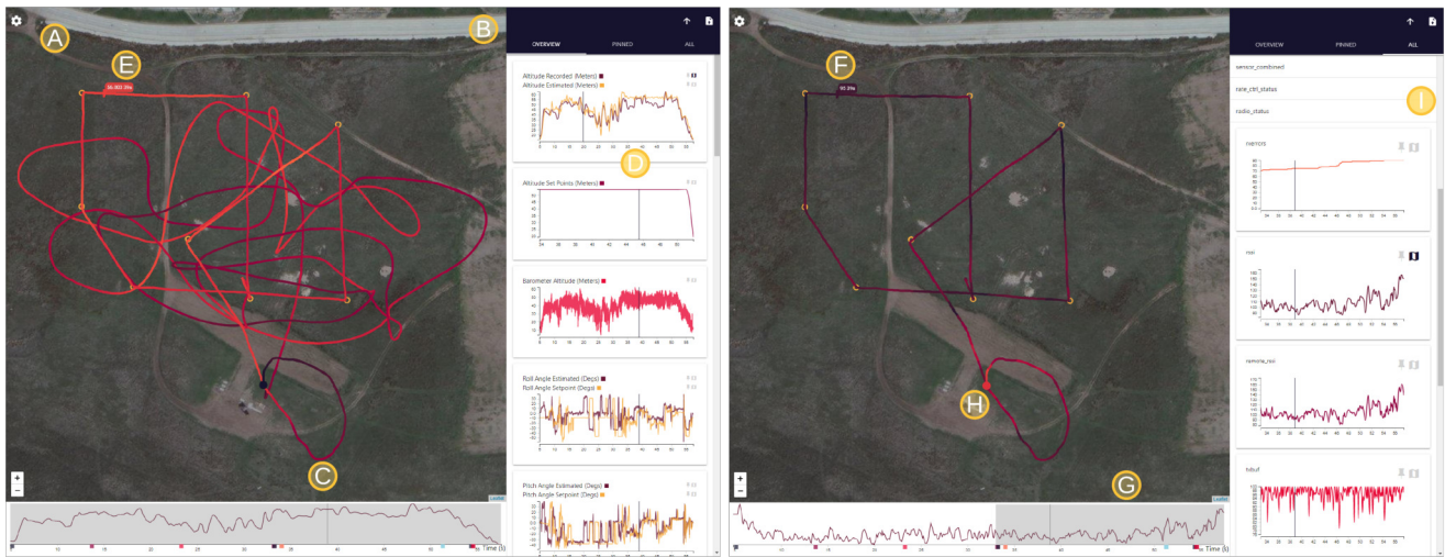
Figure 6: DATA COMETS visualizing the same flight log scene in fig. 5. All data is selected with the attribute tree displaying Overview tab (left). Data is filtered to only show data from the beginning of autonomous flight with the attribute tree displaying All tab (right). Demonstrated: (A): satellite image based map, (B): attributes tree panel displaying Overview tab, (C): timeline with all data selected, (D): line chart hover interaction, (E): flight path encoding selected attribute (altitude) with color, (F): filtered flight path with hover interaction, (G): filtered timeline, (H): glyph representing the current drone position from data selected encoding selected attribute (RSSI) with color, (I): flight message drop down elements in All tab.
