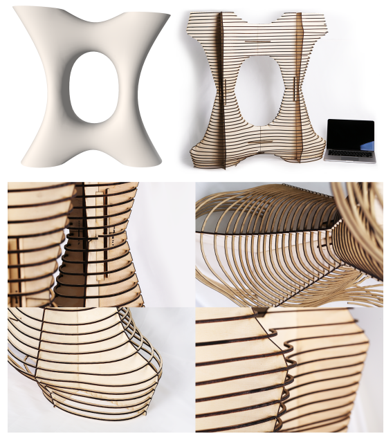
Figure 18: Here we show how our method can be used to fabricate large scale objects with holes. The object is 90 cm tall and consists of 4 springs or 8 packable parts.
