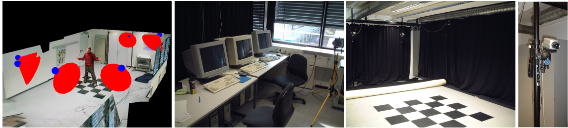
Figure 1: Illustration of the acquisition room with cameras rendered as cones (1). The control room of the studio (2) and the large recording area with calibration pattern, cameras and all-around curtain (3). One of the video cameras mounted on a pole (4).
