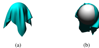
Figure 5: Cloth falling freely over a sphere with friction coefficient \mu = 0.5 : (a) using the SP method the cloth remains stable on the sphere and (b) using the PBD method the cloth falls very quickly off the sphere.
