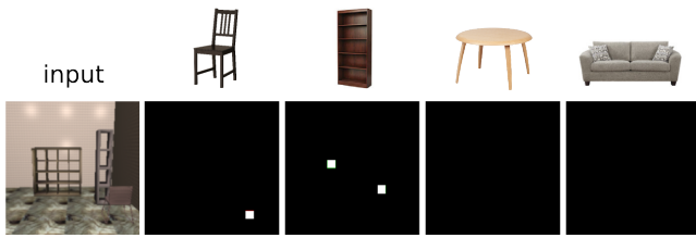
Figure 2: A scene map describes the scene on a per-class basis from a top-down view corresponding to an input RGB image. A white square indicates the presence of an instance of that particular class at that location. Here we show the groundtruth scene map, while our result can be seen in Figure 7, bottom row.
