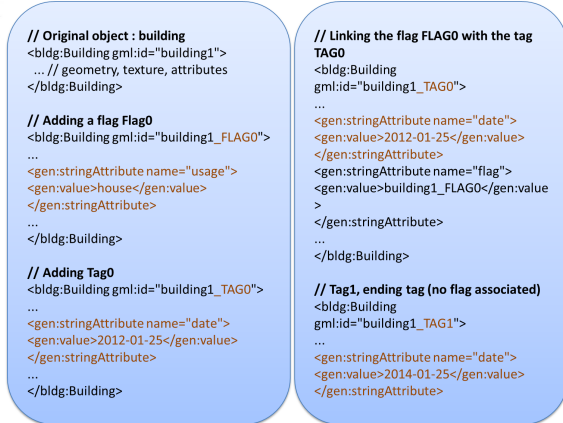
Figure 4: Tags and flags are added with modifications of IDs with suffixes and generic attributes strategy.
