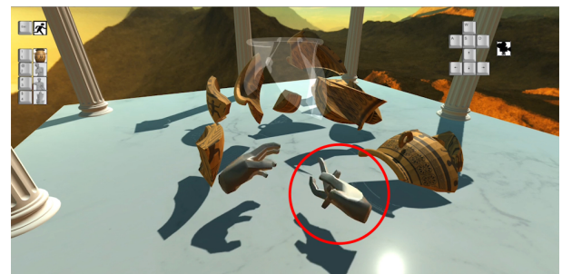
Figure 4: External directed light interference error on the Leap Motion causes tracking artifact and consequently 3D mesh screwing. This scenario provides a bad user immersion feeling feedback.
