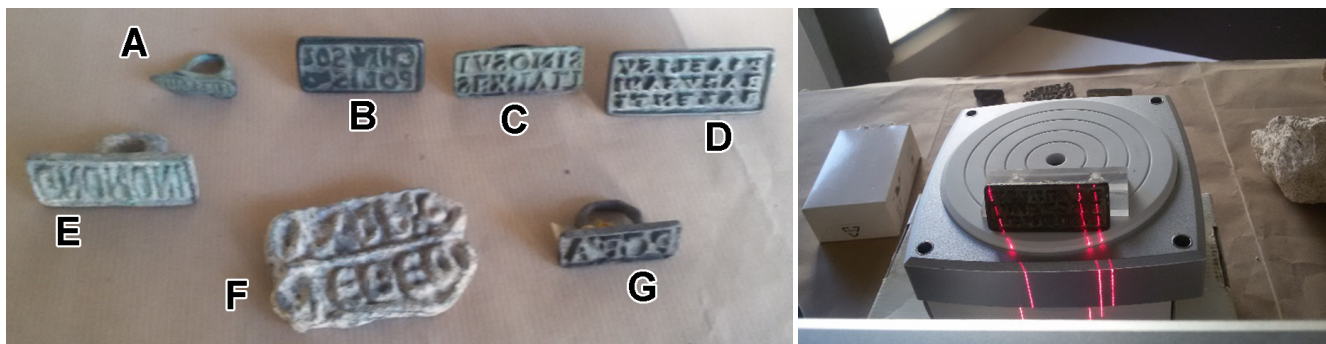
Figure 1: Group of metal signacula from the Archaeological Museum of Syracuse (on the left). Seals are identified by letters in the figure, while Inv. IDs, written within commas, are the following: A (16192), B (16191), C (33131), D (22478), E (SN1), F (SN2), and G (SN3). 3D scanning of a signaculum D via NextEngine triangulation laserscanner (on the right).
