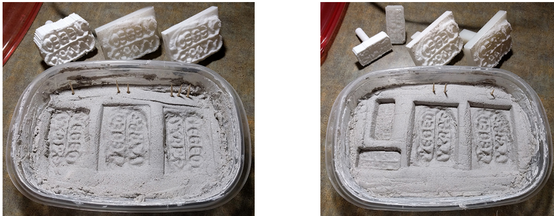
Figure 4: Cases A (shown on the left) and B (shown on the right) filled with mortar. On the upper part of the images seals are shown, while on the bottom part their related print replicas are clearly visible.
