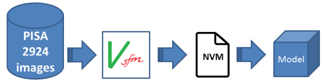
Figure 1: Initial workflow: images of a collection are processed with VSfM and a Model is obtained through parsing of the NVM file (3D reconstruction) and meta-data aggregation from our framework.
