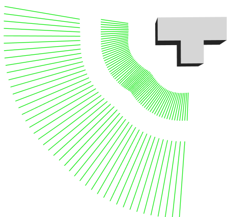
Figure 9: Eye-target camera vectors at different distances obtained using scale dependent field approximation.
