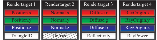
Figure 3: The layout of the G-buffers used in our method.
