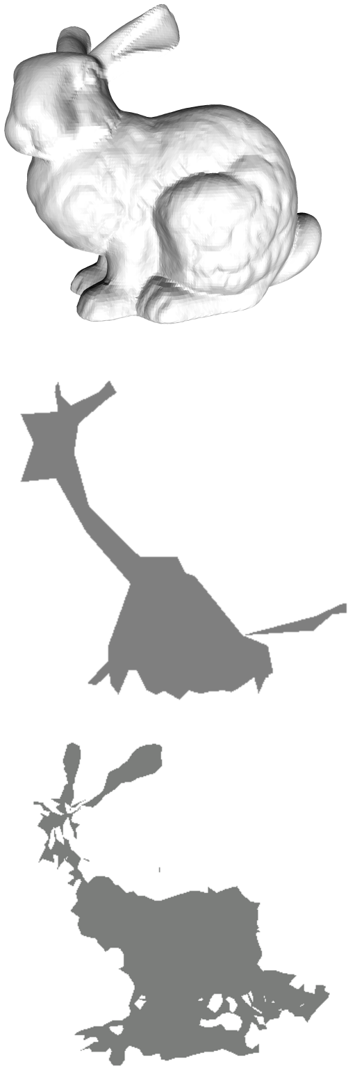
Figure 8: The Stanford Bunny (top, 69,451 triangles), its approximated medial axis (middle, computed in 17.64 seconds) and the medial axis computed by expansion of spheres with fixed radii (bottom, computed in 888.6 seconds).
